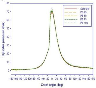
Fig.4.1: Cylinder Pressure against Crank angle
