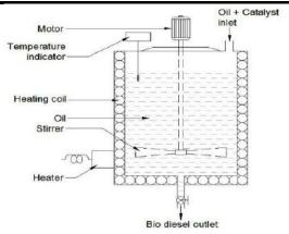
Fig.2: Schematic diagram of Biodiesel Plant
