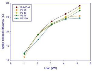
Fig .3.1 Brake Thermal Efficiency against Load
