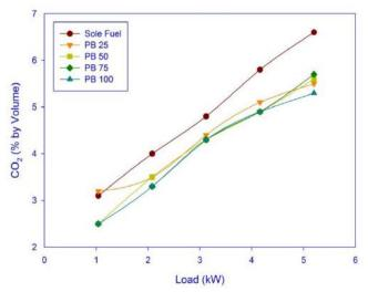
Fig.3.4: CO<sub>2</sub> against Load
