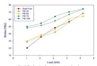
Fig.3.7: Smoke Density against Load
