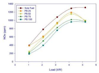
Fig.3.6: No<sub>x</sub> Emission against Load
